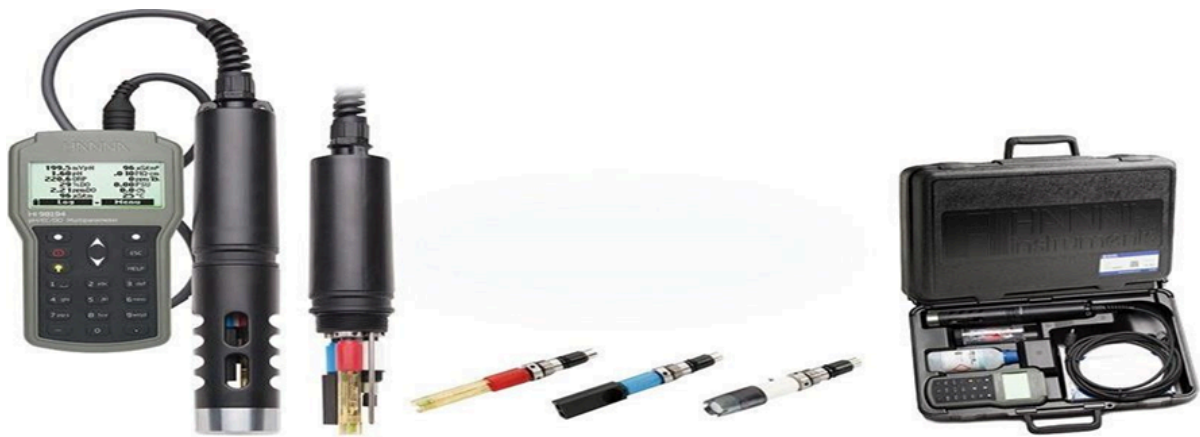
Figure 21. Technical detail for the HANNA multi-parameter probe. The key parameters measured are pH, ORP, Conductivity, Dissolved Oxygen, Temperature.
